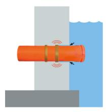
Pull off silicone paper and affix 2 rings of MASTERSTOPSK around the pipe to be waterproofed.The rings must be at least 5 cm apart.Butt joint ends, no overlaps.The surface of the pipes must be rigid.
