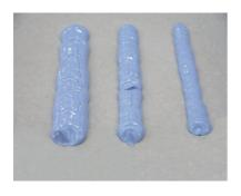
The combination of the discharge aperture and the usage volume which you can find in the technical datasheet results in the required area of application in order to guarantee professional sealing.
