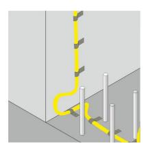
When changing between horizontal and vertical installation direction, the injection hose must be routed right into the corner of the joint and routed upwards via a loop. The minimum radius as well as the concrete cover need to be observed.
