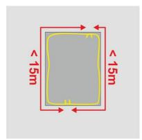
The injection hose **MASTERTUBE** "**YELLOW**" serves as internal waterproofing of construction joints. -The length of the hose sections must not exceed 15 m. Shorter injection hose sections facilitate later injection. - The injection hose is installed in the centre of the construction joint or – in case of constructional elements with a thickness of > 60 cm – at a distance of 15 cm from the water-remote side of the structure.
