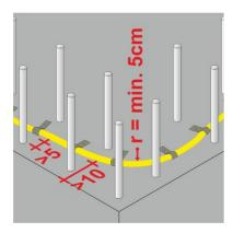
Changes of direction must be carried out with a sufficient bending radius in order to avoid damage to the hose or an obstruction of the overall injection.
