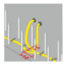
Fastening packers are screwed into the ends of the injection hose sections up to the thread end and fixed to the formwork surface. The position of the fastening packer should ensure permanent accessability (floor structure and Technical Building Equipment must be taken into consideration). The fastening packers have closure plugs in 2 different colours. These are used for marking of the pairs used for the individual hose sections.
