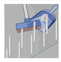
The concrete surface which the **MASTERTUBE** "**YELLOW**" is to be installed on must be as follows:
