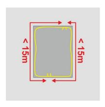
The injection hose **MASTERTUBE** "**YELLOW**" serves as internal waterproofing of construction joints.
