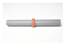
Completely mounted **ActiveRing mini/maxi**. The **ActiveRing mini** can be used for plastic distance tubes with an outer diameter of 25 - 32 mm (e.g. plastic distance tubes 22/26, 26/31 und 26/32). The **ActiveRing maxi** can be used for fibre cement distance tubes with an outer diameter of 38 - 42 mm.
