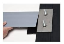
The joint sheet metal to be connected is now overlapped by 5 cm with the coated side (complete length) of the **joint sheet metal/joint tape connector**.
