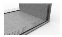
Installation of the **SFE profile** is complete; the next cavity wall element can be placed.
