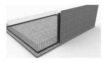
Installation of the **SRF profile** is complete; the next cavity wall element can be placed.
