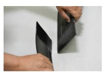
Press both ends, one prepared with MMF 140 adhesive tape, one without adhesive tape, together and bond them.
