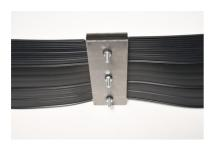
Use a torque wrench to tighten the bolts to 8 Nm torque
