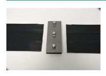
Remove the horizontal waterstops (ribs) on both sides, at the front and back to the depth of insertion using a sharp utility knife.
