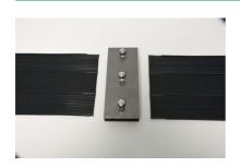
Insert the two ends of the joint tape into the MASTER-Connect joint tape connector until they are touching the bolts.
