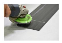
Grind down the corrugations in the bonding area with a grinding disk.
