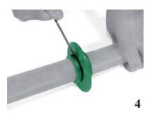
Tighten both fastening straps by hand
