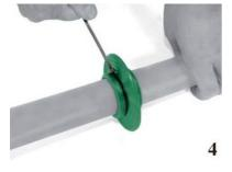
Tighten both fastening straps by hand
