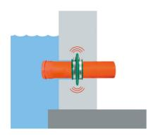
Der **RONDO Sealing collar** is positioned in the center of the concrete component.
