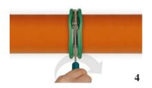
The clamping strap is tightened to approx. 5-6 Nm torque to prevent the **RONDO Base** from shifting during concreting.
