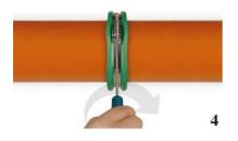
The clamping strap is tightened to approx. 5-6 Nm torque to prevent the **RONDO Base** from shifting during concreting.
