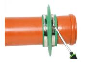
Apply lubricant to the clamping range of the strap, then tighten the clamping straps sufficiently using a screwdriver to prevent the **RONDO sealing collar** from shifting.
