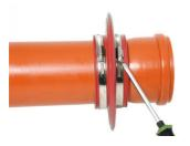
Apply lubricant to the clamping range of the strap, then tighten the clamping straps sufficiently using a screwdriver to prevent the **RONDO Protect sealing collar** from shifting.
