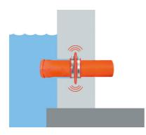
Der **RONDO Protect Sealing collar** is positioned in the center of the concrete component. It reliably and permanently prevents water penetration at the outer pipe wall.
