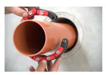
When using a **MASTER-SEAL** modular seal in combination with an existing installation, the "open" modular seal is placed around the existing medium pipe and closed as described at the beginning. Proceed as shown above.
