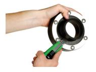
Cut off the pushed-through ring using a cutter – the gasket is now ready for installation.
