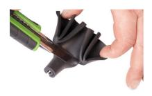
Pull out the ring segment you want to remove and sever it with a cutter.
