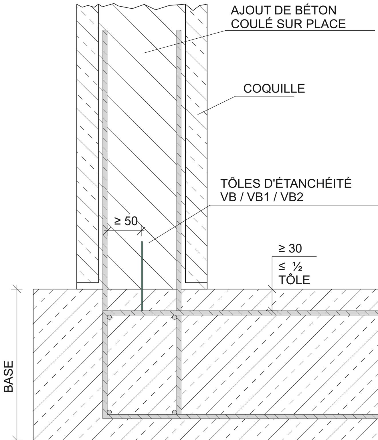
POUR LES TÔLES REVÊTUES D'UN CÔTÉ, LE REVÊTEMENT DOIT TOUJOURS SE TROUVER CÔTÉ EAU.
